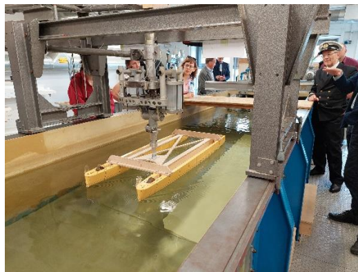
Figure 4. Wave lab at university of applied sciences in Kiel with a model of a autonomous ferry by CAPTN.
