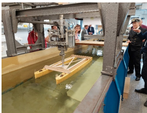
Wave lab at university of applied sciences in Kiel with a model of a autonomous ferry by CAPTN.
